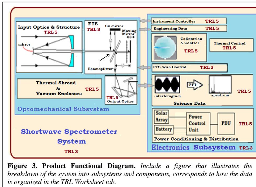
Figure 3. Product Functional Diagram. Include a figure that illustrates the breakdown of the system into subsystems and components, corresponds to how the data is organized in the TRL Worksheet tab.
